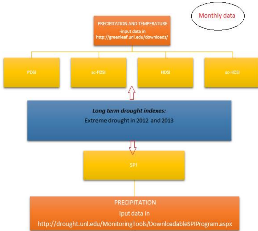
Figure 66: Long-term drought indices. Monthly mean precipitation and monthly mean temperature from 1980 to 2013 are the input data used to calculate PDSI, sc-PDSI, HDSI and sc-HDSI. Monthly mean precipitation is the input data to calculate SPI. All the mentioned indexes show extreme drought periods in 2012 and 2013.
